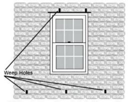
Weep holes allow air into the cavity and moisture to drain out
